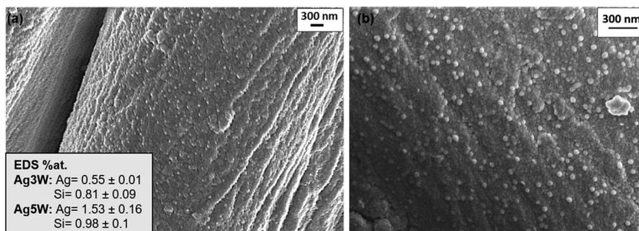
**Fig. 2.** Typical morphology (FESEM images) of the coated mask (Ag3W) at lower (a) and higher (b) magnification: bright spots are silver nanoclusters embedded in the silica matrix. Coated textile fibres are visible, with the EDS analysis in at% of Si and Ag relative to the two coatings (Ag3W and Ag5W).
